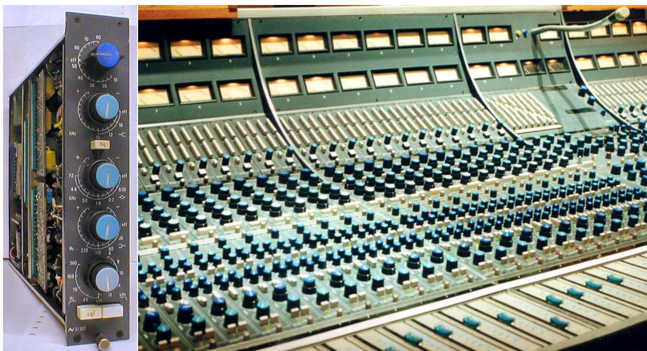
One Neve 31102 EQ hardware module and 31102s installed in a Neve 8068 console
