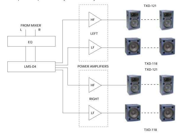
Tri-amplified live performance system of two-way enclosures with subs
