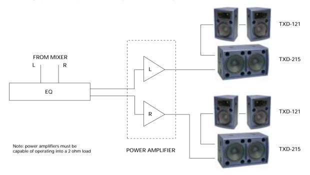
Bi-amplified live performance system of two-way enclosures with subs
