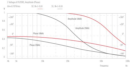
This plot shows the actual measured phase error for two different loudspeaker systems. One system has an upper end roll off at 20kHz while the other extends on out to a 54kHz roll off. There is clearly less phase error in the latter case, not just at high frequencies, but also well within the accepted range of human hearing where harmonic recognition starts as low as 5kHz.
