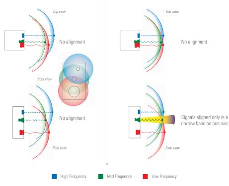
In a Dual Concentric driver the signal sources are perfectly aligned, resulting in smooth response and a wide listening area in both horizontal and vertical axes.
