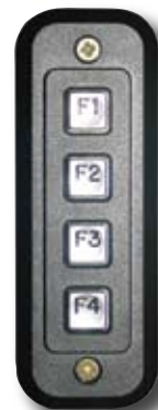
Example of control panel using the external I/O ports
