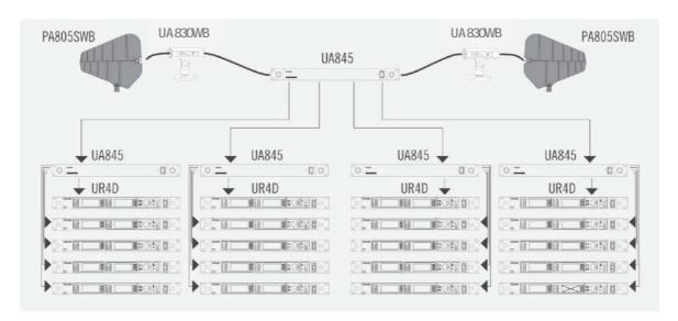
A 40 channel system (**UHF-R cascading**) requires only 1 x UA845, but requires that a stack of cascaded receivers are of the same frequency band version because of the Track Tuning Filter capability of the UR4:
