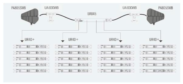
Please note that the RF cascading (active circuitry) only works if the respective receiver unit is powered on.
