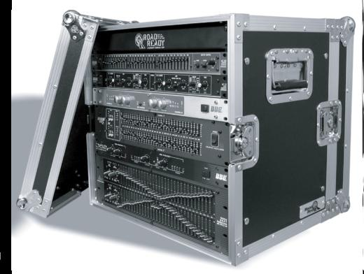
Built smart with flexibility and comfort in mind, the RR10UED accommodates professional effects units up to 10U. This rugged case is designed to fit all standard 19" rack-mountable equipment, features dual rack rails (mounted front and back at a 12 3/8" rack depth) and includes two removable covers for easy access to both sides of your rack. Built for the long haul!
