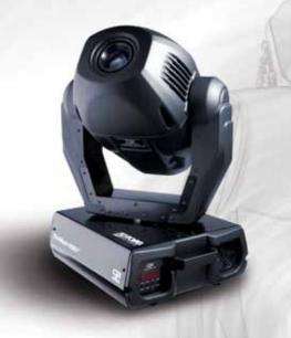
The ClubSpot 500 CT offers colour wheel with 9 dichroic filters; rotating gobo wheel with 6 rotating, indexable and replaceable gobos; 3-facet prism and 2 manual adjustable beam apertures 15° and 22°. This fixture is ideal for middle installation applications.
