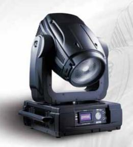
The ColorWash 700E AT is the first Wash fixture using the MSR GOLD 700 FastFit lamp in the Robe range. This powerful moving head offers a full CMY + CTO colour mixing system, a colour wheel with 7 replaceable "SLOT&LOCK" dichroic filters, a rotating beam shaper and a linear zoom range of 6° - 45°.
