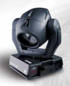
The ClubWash 300 CT includes a 250W discharge lamp, high luminous efficiency parabolic reflector, CMY colour mixing, colour wheel with 6 dichroic filters plus open, smooth dimmer and silent fans for cooling. The fixture is perfect for small to medium installation applications.
