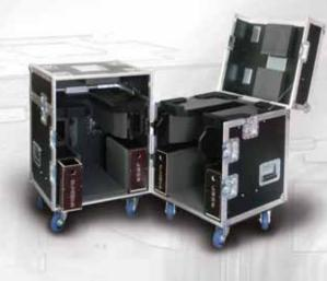
The Dual 575 Touring Case provides full protection for the moving heads in the 575 series during transportation and touring. It was designed to endure the rigors of the touring and rental market. The case is manufactured from high-quality, water repellent 13mm thick plywood. It has a black finished exterior and features aluminium protected edges and tough steel corners. Roller castors on the base enable easy roll-on and roll-out.
