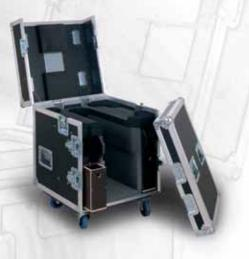
This case provides perfect protection for Robe's DigitalSpot 3000 DT in the touring and rental market. It is constructed from high-quality, water repellent 13mm thick plywood. It has a black finish exterior and features aluminium protected edges and tough steel corners. This single case is equipped with four metal recessed wheels for easy transport.
