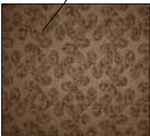
Birch plywood, special water resistant quality, anti skidding top layer
