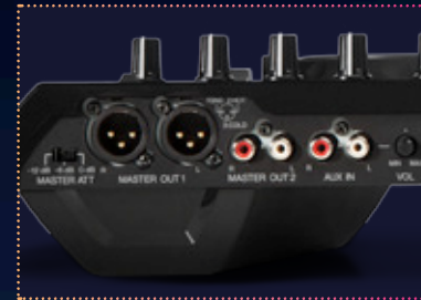
Multiple inputs and outputs Including a balanced XLR input and output for direct connection to PA system with no loss of sound quality.
