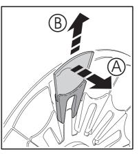
Figure 7: Filter replacement
