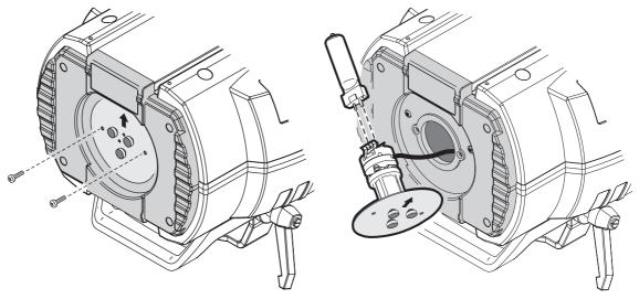
Figure 1: Lamp installation
