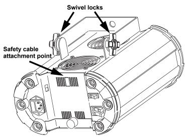
7 Verify that the fixture is at least 1 meters (3.3 ft.) from the surface to be illuminated and at least 0.3 meters (1 ft.) from any combustible materials. Verify that the clearance around the air vents is at least 0.1 meters (4 in.).
