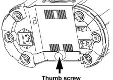
3 Slide the fixture cover open as far as possible (there is a physical stop point that prevents access to the power supply section).
