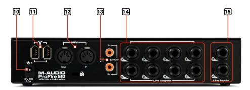
10. **Power Input ( - + ) -** Connect the 12VDC 2A power supply here when using ProFire 610 with a four-pin FireWire connection, or if your computer does not provide sufficient bus power on a 6-pin connection. If your computer can provide power over a 6-pin connection, it is not necessary to use the included power supply.
