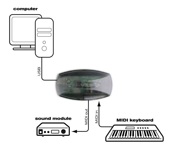
In the set-up described above, MIDISPORT 1x1 is being used to route MIDI data between the controller keyboard, the sound module, and the computer. To set up MIDISPORT 1x1 in this way:
