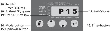
Fig. 1: Adjusting the pump output
