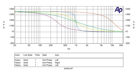
Response of the all pass filter for 2nd order phase shift with Q=1 at frequencies of 300Hz, 1kHz and 10kHz and also with Q=6 at (max) and Q=0.4 (min) at 1kHz
