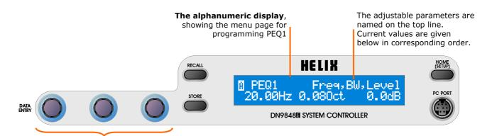
**DATA ENTRY control knobs** adjust the left, centre and right parameter values at the display, in corresponding order. If there are only one or two parameters, only the active controls are lit.
