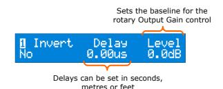
the Level is set to 6dB, the 0 represents 6dB. Turning the rotary Gain Control right/left will increase/decrease the level in a proportional manner beyond 6dB (it is not directly additive since the gain is limited to +12dB). Hence, the Output Gain controls enable fine-tuning during a performance, while the baseline output level is retained as a standard setting for future use.
