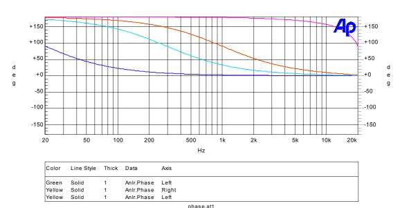
Response of the phase shifter filter for a phase shift of 90° at reference points equivalent to 20Hz, 300Hz, 1kHz and 20kHz
