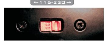
The device is default set to be connected to 230 V AC Power. To use the device on a 115 VAC Power you need, before connecting it, to move the voltage selector's cover, just loosening the two screws, and to choose the correct use voltage by the red switch. Be sure that both voltage set on the selector and AC Power have the same value . Always close the voltage selector's cover before connecting the device to AC Power. Change the label that points out the correct voltage in use.
