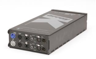
The K-array KA line of power amplifiers are built into a 2U, half-rack, light weight aluminum chassis. Each model is comprised of two or four output channels providing up to eight channels in a standard 2U rack space when mounted together. KA amplifiers feature optical limiters, and protection against over temperature, over current and short circuits.
