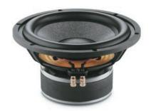
"W" cone, high excursion Focal 11W7670 11" driver unit included in the Sub6. Featuring a 2.6" voice coil diameter and a 1.6" high, 6.25" diameter dual ferrite. Optimized gap with extended pole piece for very symmetrical field and reduced distortion. Heavy duty spider and surround. Driver's weight: 8kg...
