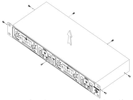
Removing seven screws to access internal fuse
