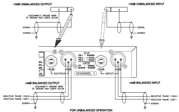
CONNECT NEGATIVE PHASES (PIN 3) TO GROUND (PIN 1) IN EACH XLR -
