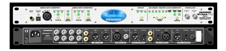
M-Clock Plus is a high stability master clock generator offering clock rates between 44.1 and 192kHz. In addition to the internal clock source, the M-Clock Plus can distribute an external word clock source or extract the clock frequency from an AES11 (digital black) source.
