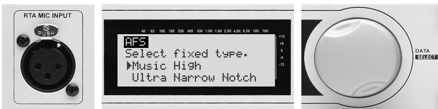
34A - Using the Data Wheel, choose the EQ notch filter width appropriate for your needs. Speech is a wide filter, Music Low is a narrow filter, Music Medium is a Very Narrow filter, and Music High is an Ultra Narrow filter (Music High Typical).
