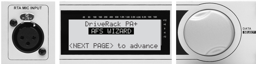
31A - The first screen of the AFS Wizard appears on the display.
