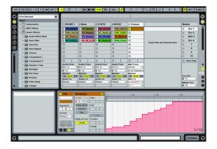
The Live set we created contains 4 audio tracks each with 4 clips in it. Each of the 16 combinations of the faces of the Sender – Receiver cube pair corresponds to one of the audio clips.
