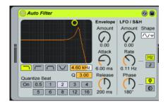
This effect will filter out certain frequencies of the sound while we are playing it back. Let's say we want to change the frequency above which the sound is attenuated (lowered in volume), called the cutoff frequency.
