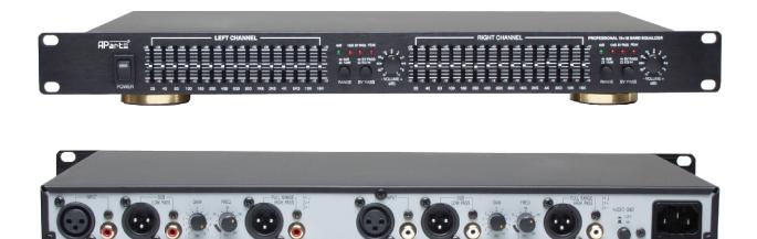
The Apart PXQ2215 looks like a standard 2 x 15 band EQ, but in real it is much more than that. The PXQ2215 combines the EQ section with a 2 way adjustable X-over at the back. Turning the frequency pot-meter completely to the left, results in a Full range output.
