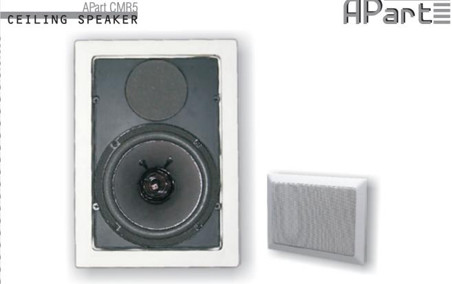
The APart CMR5 is a neutral rectangular 100 volt built-in speaker, provided with a 5.25" dual cone woofer. Due to its clear sound reproduction, the CMR5 is very suitable for the distribution of backgroundmusic and microphone calls. This loudspeaker has a 100 Volt 6 watt transformer with several power tappings.
