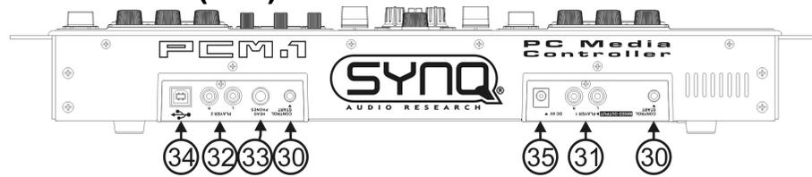
30. **FADER START:** when used with an external mixer you can connect this output with the fader start input of your mixer to control the start/stop function of the player from your mixer. (**attention:** works only with Pioneer®/SynQ® compatible mixer)
