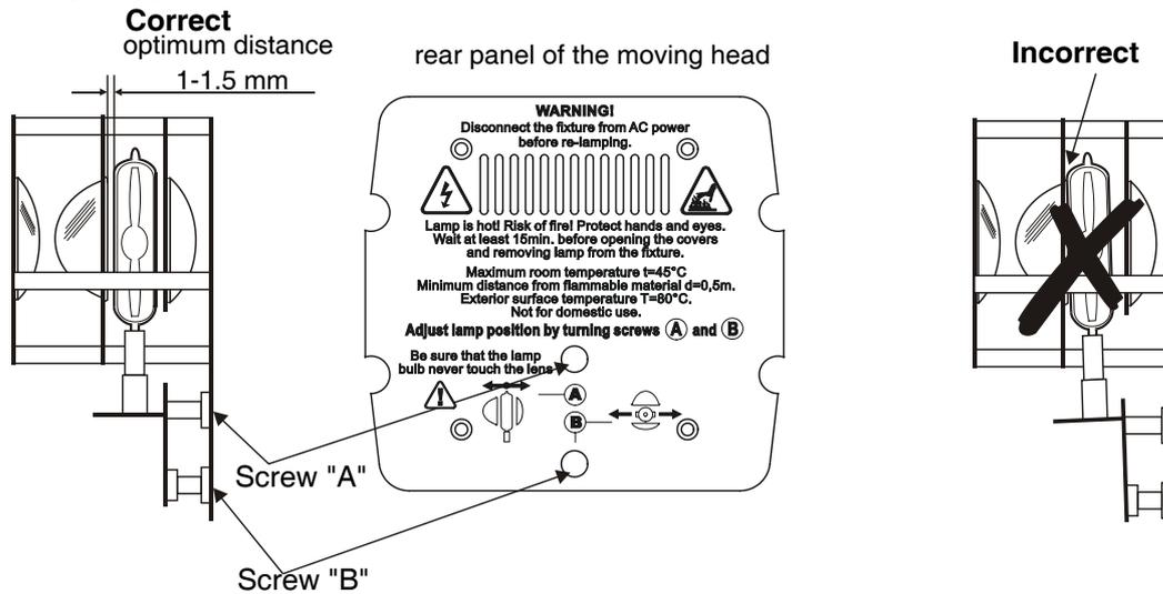
The lampholder is aligned at the factory. Due to differences between lamps, fine adjustment may improve light performance.
