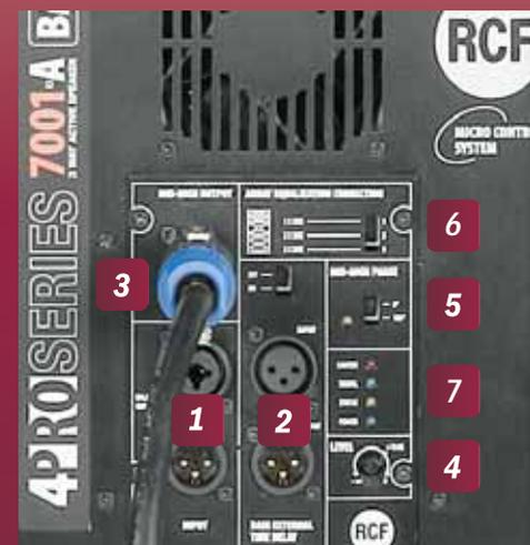
The very unique input section presents a combo XLR/Jack line input connector, a recessed master volume and a useful XLR loop-through link. Extra features are the Bass external time delay in/out, the "3-position" array equalisation, the mid-high phase switch.
