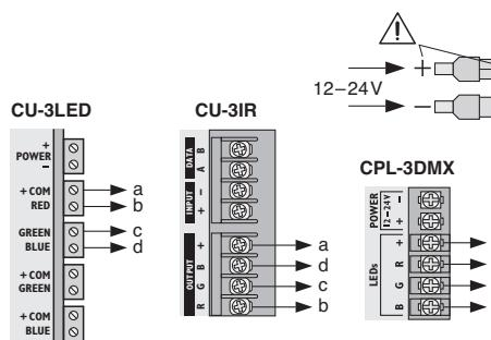
To facilitate connection, all terminals can be removed.
