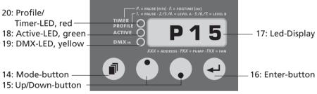
Fig. 1: Adjusting the pump output
