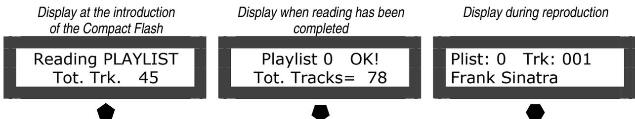
At the end of the reading operation, if the names of the pieces have been fitted in correctly, Replay will automatically starts to reproduce the musical items in the programmed sequence.
