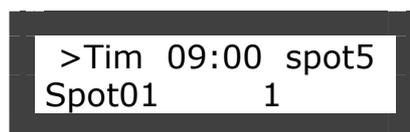
Select the bar to display using the ENTER key, use the keys < or > to show how many spots make up the bar, and the names of the spots.
