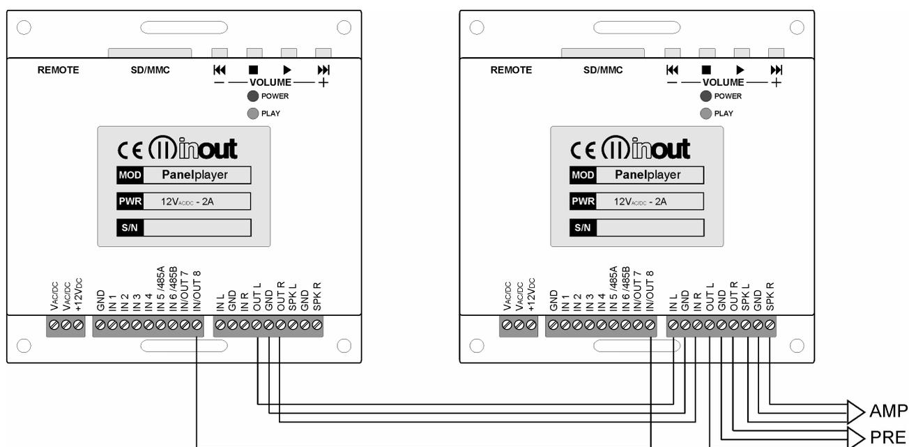
When an hour bar is to be played, the schedule-programmed Panelplayer waits for consent for the end of the item from playlist-programmed Panelplayer (which goes into standby), before starting to issue the commercials. Once the playing of the hour bar is over, the playlist-programmed Panelplayer will start to play the following item.
