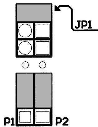
Position **P1** and **P2** jumpers: IN5 and IN 6 inputs enabled to the operation as RS485 serial port. To move the bridges, raise the cover of the device and move the jumpers of the board as indicated in the figure.
