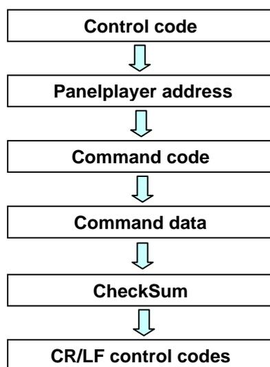
**! IMPORTANT:** the introduction of **CheckSum** at the end of the block of data and characters of **CR + LF** is defined in the configuration file (par. 9.2).
