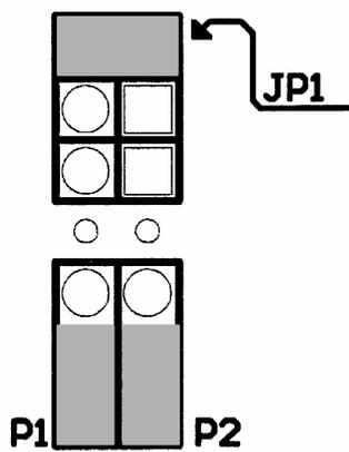
Position **P1** and **P2** jumpers: IN5 and IN6 inputs with logical operation. (*Default*)
