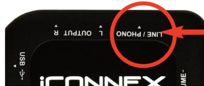
Make sure the input select switch is set to the input you are using.
