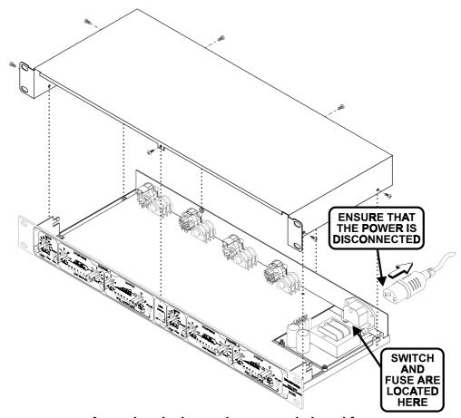
Accessing the internal power switch and fuse
