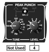
Filter section (TUNE) is not used in FULL BAND mode.
