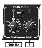
Using the filter to TUNE the punch.
