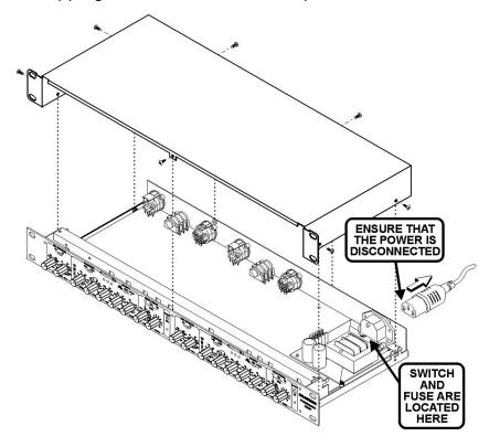
Accessing the internal power switch and fuse
