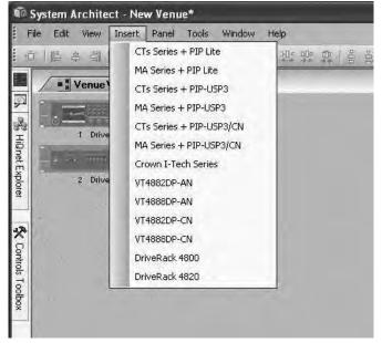
The Insert Menu provides the ability to insert devices into a venue.
