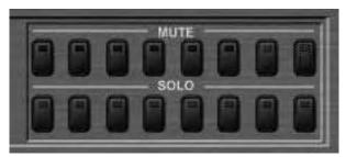
The Mutes and Solos are also in the bottom left hand corner of the Device Window, directly below the Meters. Mutes provide a quick way of muting DriveRack 4800 outputs. The Solos employ the Mutes for soloing of a single channel during setup.
