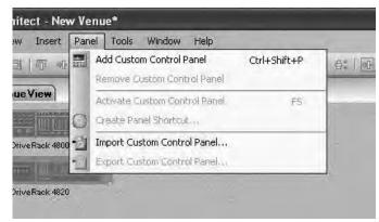
The Panel Menu option lets you create and manage Custom Control Panels, with functions including add, remove, import, export and activate a control panel.
