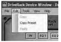
In the Device Edit Menu you can Copy and Paste processing module parameters as well as the Preset.
