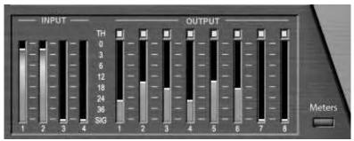
The Meters in the lower left hand corner of the Device View are real time meters, and they show the current input and output levels if the unit is online. The meters can be turned off to reduce the amount of network traffic if so desired.
