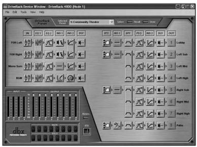
The DriveRack Device View (seen below) is accessed by double-clicking the device icons in System Architect's Venue View, and provides access to the processing modules and other features of the DriveRack 4800 or 4820 devices. Like the processing icons, the device icons look like the devices they represent.
