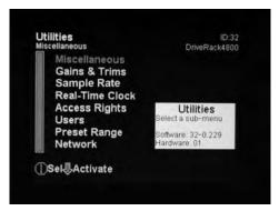
**Page Navigation** - This is the easiest and most common type of navigation within the DriveRack 4800. Page navigation is used when there are several pages of parameters that need to be accessed. An example of Page navigation is found in the Compressor editor where there are three pages of parameters and the NEXT and PREV PAGE buttons are used to move between these pages.
