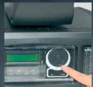
2x16ch LCD display with easy jog wheel navigation
