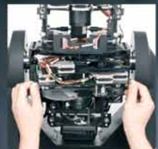
Easy servicing and motorized linear zoom 15°-35°
