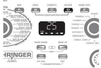
In this case, pressing button A, B, C or E will call up another preset within bank 25. The two arrow buttons (BANK UP and BANK DOWN) enable you to change banks. The display will show which bank has been selected, but the preset will not change until you press one of the A – E buttons. The LED beneath the preset letter lights up when that preset is activated.
