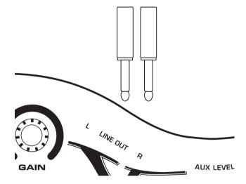
20. LINE OUT – Plug balanced or unbalanced ¼" cables into these jacks to send the stereo signal for recording or performance applications.
