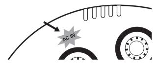
AC IN – Plug the included power cable into this socket. When connected to the mains, the V-AMP 3 switches on automatically.
