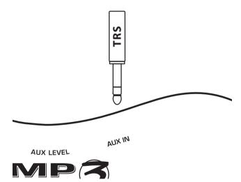
AUX IN – Plug an external sound source into this jack using a ¼"TS or TRS cable.
